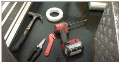
Typical tools for sarking tied roofs
