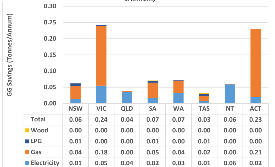
Figure 19: Household level greenhouse gas savings – Top-up ceiling insulation (t CO 2-e /annum)
